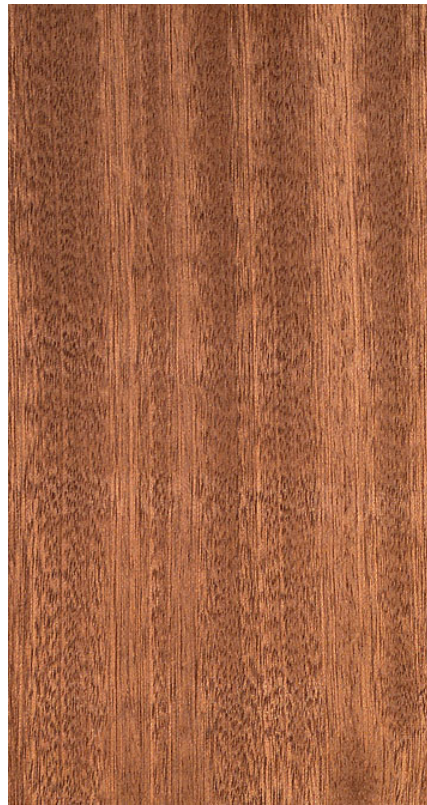
Wood surface of Sapeli (radial section)
