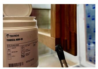
Teknoseal 4000 applied by brush to exposed end grain prior to factory finishing
