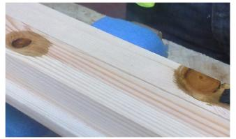
The area in and around knots needs particular attention, due to the high density of the knots and levels of resin they contain. Preservative treatment partially dissolves and mobilises resins which are drawn out towards the timber surface as the solvent evaporates. In most cases this occurs before the joinery is factory coated. However, around resinous knots/timber, if insufficient drying time
