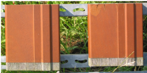
After 24 months exposure, moisture ingress on the untreated end grain on the top of the right hand component has caused splitting, discolouration and adhesive failure at the cut edge.
