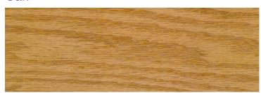
Oak is a durable Northern Hemisphere timber widely used for timber frames, garden furniture and, less commonly, windows, doors, and conservatories. The species typically used are European Oak and American White Oak. Oak contains extractives that inhibit coating adhesion and should be degreased with a sharp solvent such as TEKNOSOLV 7012 prior to coating.
