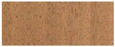
Iroko is a durable African hardwood with excellent weathering properties. Untreated, the surface turns silvery grey colour. Due to its durability, Iroko is often used for cill components in door and window frames. Iroko contains extractives, which can prevent good adhesion of surface coatings, and surfaces should be degreased with a sharp solvent such as TEKNOSOLV 7012 prior to coating. Cloths used to apply solvent should be replaced regularly to avoid spreading resin across the surface.
