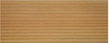
European Redwood is the most common timber used in window and door production, but due to its durability class, it must be preservative treated to hazard class 3, BS EN 335-1.
