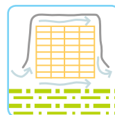
Ventilation under presenning
