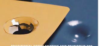
TRADITIONAL EPOXY COATING AND TEKNOPUR 300 AFTER IMPACT RESISTANCE TEST AT -20°C.
