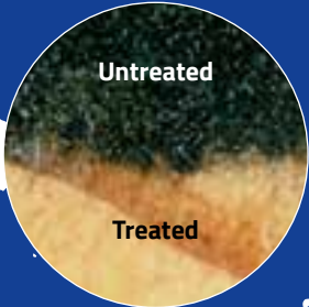
Comparison clearly shows the difference between untreated wood and wood treated against wood discoloration and wood destroying fungi.
