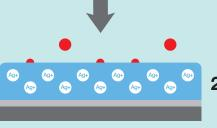
Biora Clean's antimicrobial characteristic increases the hygiene level of indoor spaces by reducing the level of microbes on the painted surface. The active ingredient is silver. The paint film retains its antimicrobial property throughout its lifespan. The product's antimicrobial efficiency has been tested according to standard ISO 22196.
