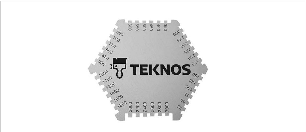
**Image 7.11** Comb-type wet film thickness metering device. The measurement is read from the furthestmost tooth coming into contact with the paint when the comb is pressed through the paint film so that the first and last tooth come into contact with the substrate.
