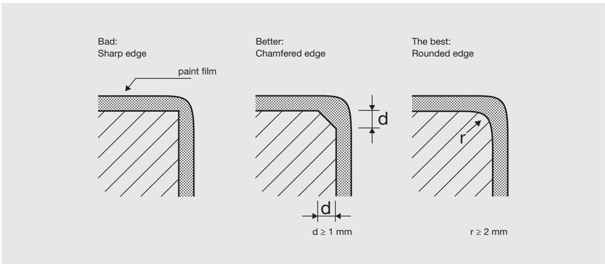
**Image 3.2** In terms of painting, rounded corners and edges are ideal, since coating thickness is uniform (ISO 12944-3). Sharp corners are to be avoided.
