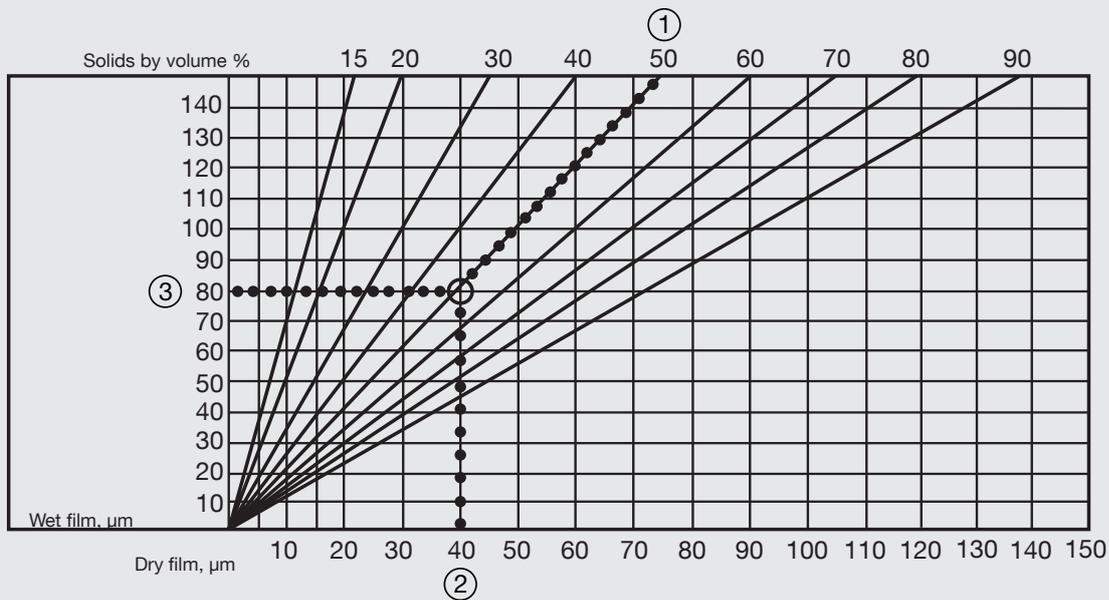
Traversal lines represent examples of the solids by volume. Start from the top of the relevant solids by volume. Follow the line downward until it meets the vertical line representing the required dry film thickness (at the bottom). Then, from the point where the traversal and vertical lines meet, follow the horizontal line to the left-hand side and read the value that corresponds to the required dry film thickness.
