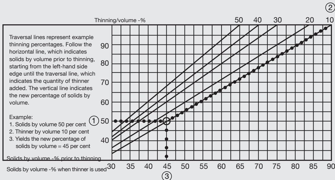
Traversal lines represent example thinning percentages. Follow the horizontal line, which indicates solids by volume prior to thinning, starting from the left-hand side edge until the traversal line, which indicates the quantity of thinner added. The vertical line indicates the new percentage of solids by volume.
