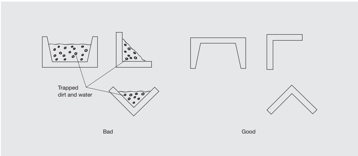
**Image 3.1** On the left-hand side, examples of structures not suitable for corrosion protection painting. On the right-hand side, examples of suitable solutions (ISO 12944-3).
