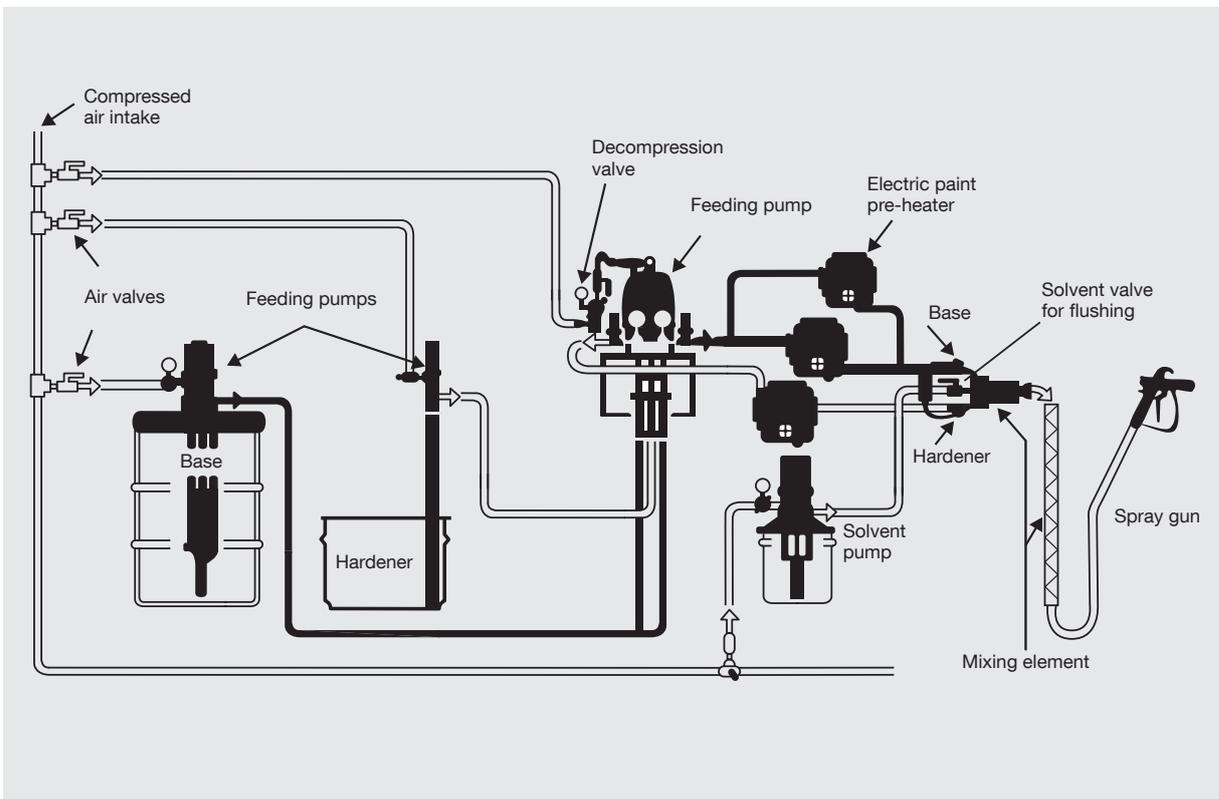
Image 7.6 Operation principle of two-pack sprayer.
