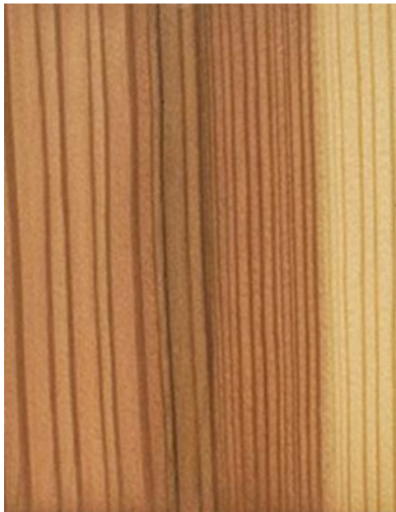
Wood surface of larch (radial section)
