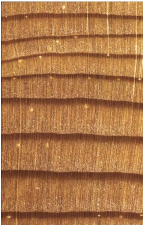
Macroscopic cross-section of larch (10 times magnification lens)
