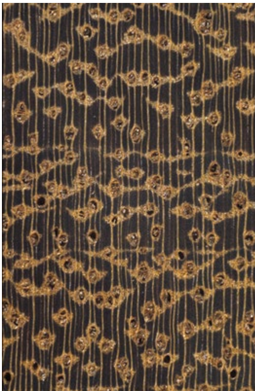
Macroscopic cross-section of Iroko (10 times magnification lens)
