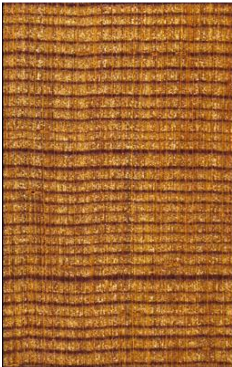
Macroscopic cross-section of Douglas Fir (10 times magnification lens)
