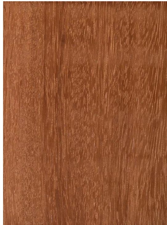
Wood surface of Afzelia (radial section)
