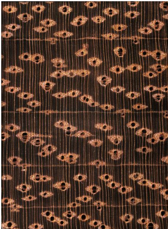
Macroscopic cross-section of Afzelia (10 times magnification lens)
