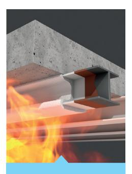
The foam insulant forms (intumescent) under the action of fire. This foam slows the passage of heat defined for each of the fire resistance classes.
