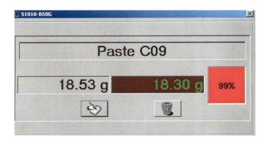
When the target weight is reached, the percentage changes to a stop sign.
