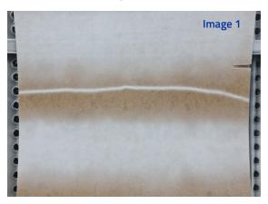
Regular quality control checks of tips for optimum performance. Every 2-3 weeks, check the tip quality for wear and tear, against the spray template from a new tip.
