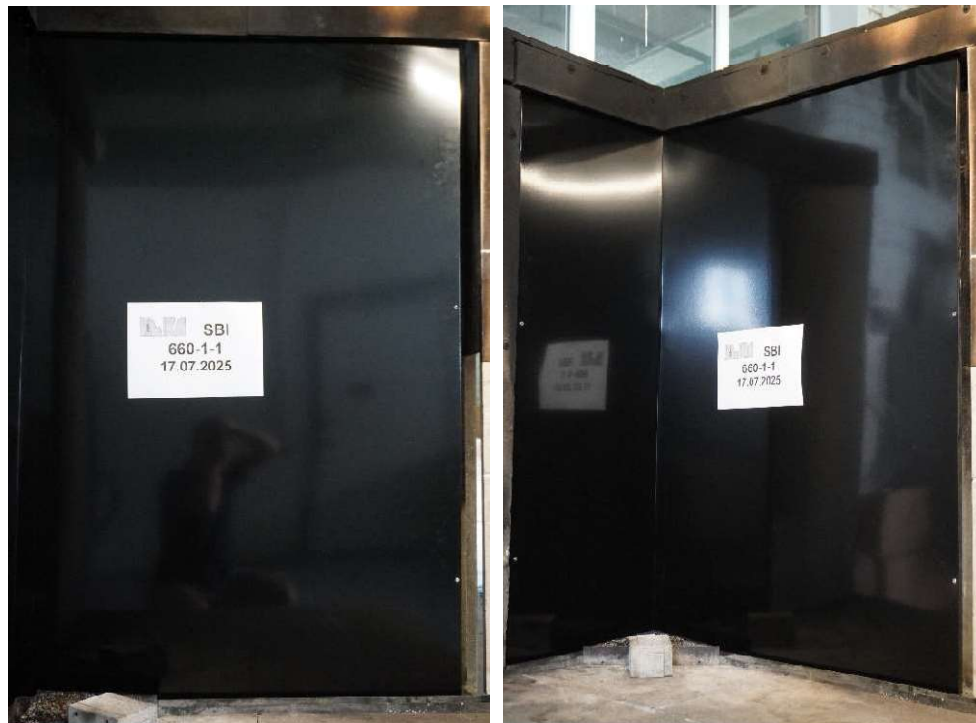
Fig. 1 Specimen mounting in SBI.
