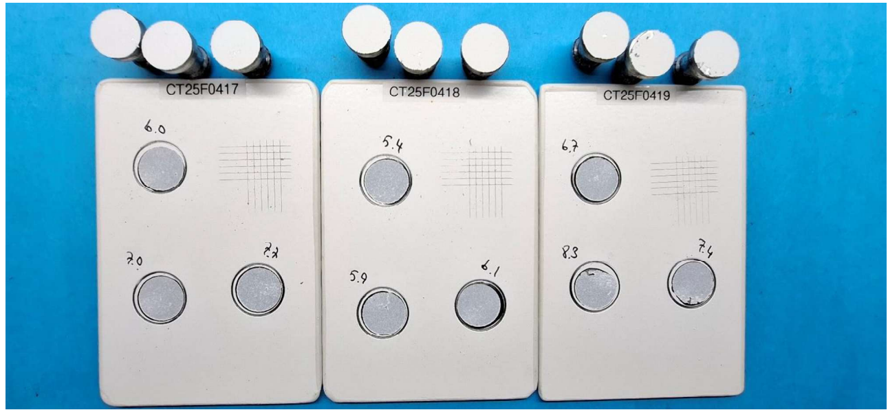
Picture 3. Condensation test panels.
