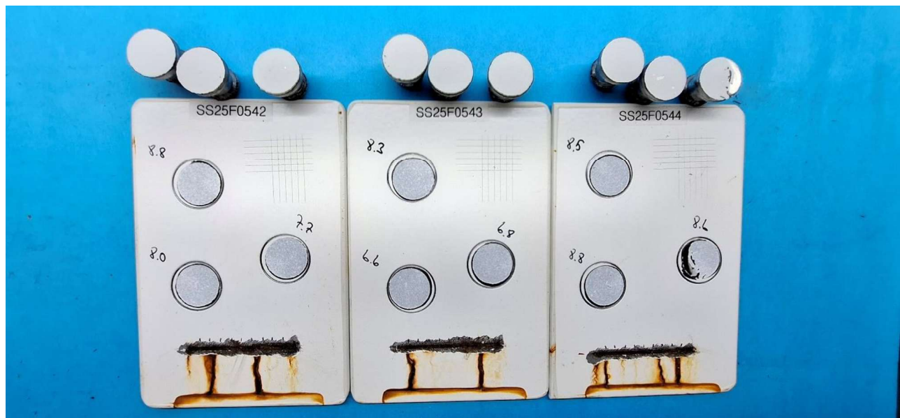
Picture 2. Neutral Saltspray test panels.
