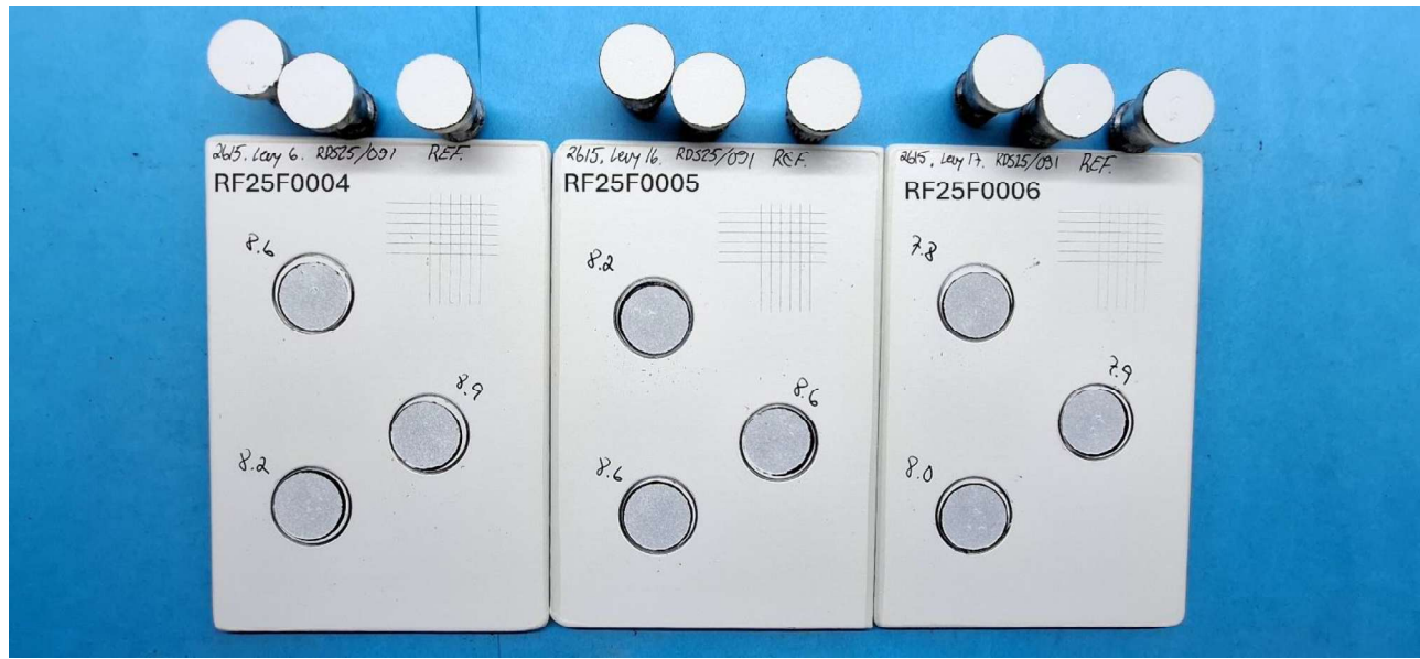
Picture 1. Adhesion reference panels.
