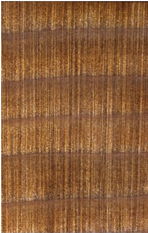
Macroscopic cross-section of Western Red Cedar (10 times magnification lens)
