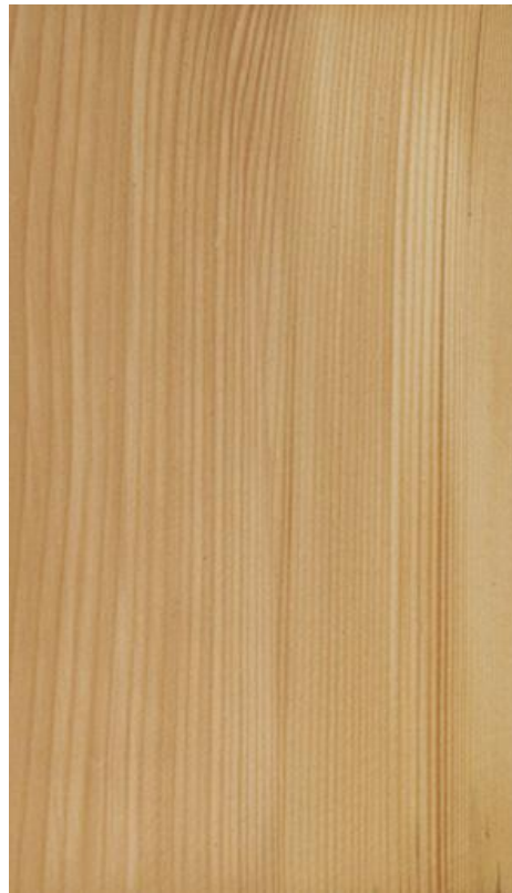
Wood surface of Silver Fir (radial section)
