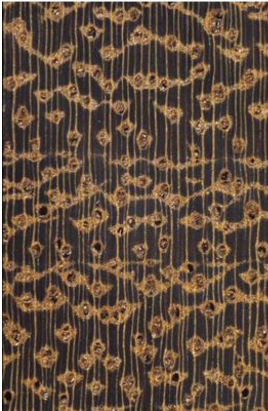
Macroscopic cross-section of Iroko (10 times magnification lens)
