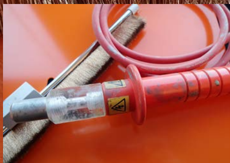
Porosity test can be used to check for pinholes, or minimum coating thickness in order to prevent early breakdown on the coating system.
