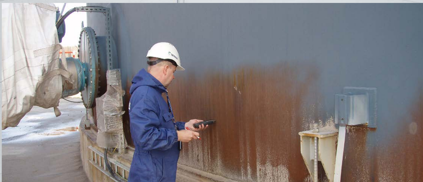
Measuring the surface temperature from the wall of a container.
