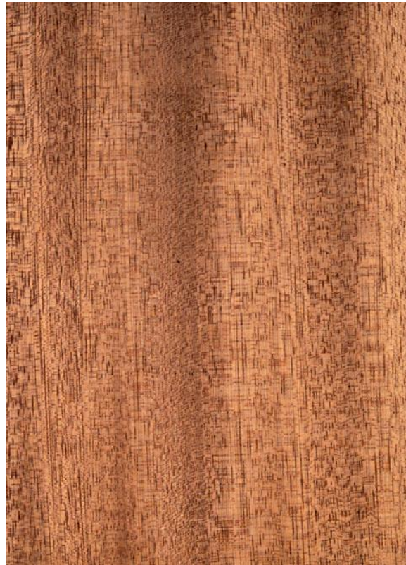
Wood surface of Sipo (radial section)
