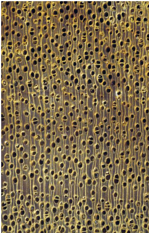
Macroscopic cross-section of Framiré (10 times magnification lens)
