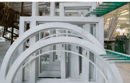
Teknos coatings resist blocking for easy handling and fast production
