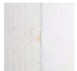
▲ The white-coated pine on the left was treated with a conventional primer while on the right it was coated with Teknos' knot sealing primer
